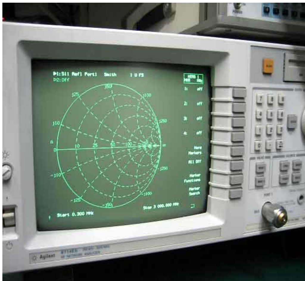
S11 50 \Omega load measurement on the Smith Chart display / Scale 1
