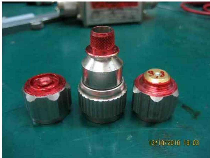
Homebrew calibration standard built by 7X2RF (left to right : Short, Open, Load).
